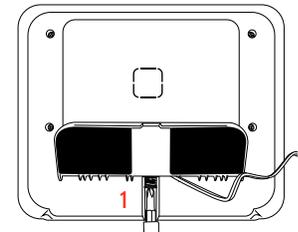
1. With a small Phillips screwdriver, screw in the locking screw from the bottom of the panel to secure it to the table stand.
