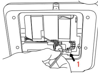
1. With the included power supply and cable, plug the barrel connector into the barrel jack as shown above.
