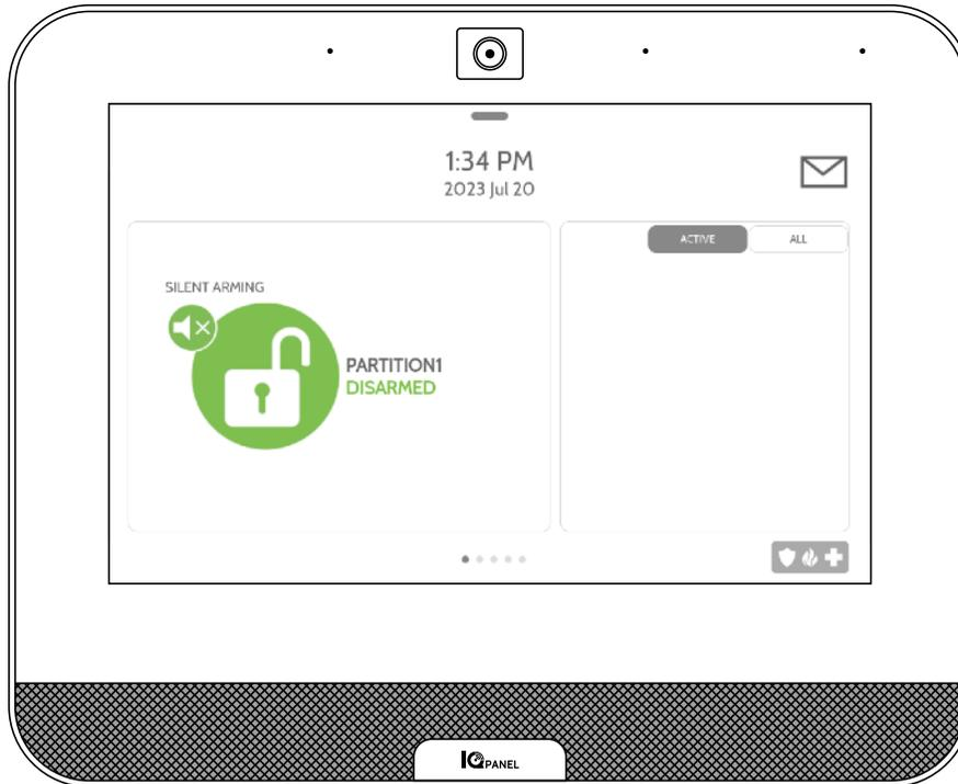
The IQ Panel 4 is an All-In-One 7" (17.8cm) touchscreen built with a built-in camera, providing full security and smart home functionality in an easy to use interface.
