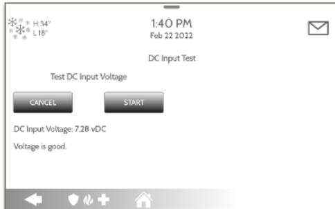
Press “Start” to run a real-time voltage test on the Panel. If voltage received is above 6vDC, you will get a “Voltage is Good” message.
