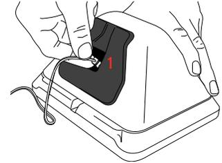
1. With the included power supply and cable, plug the barrel connector into the barrel jack on the bottom of the IQ Base as shown above.
