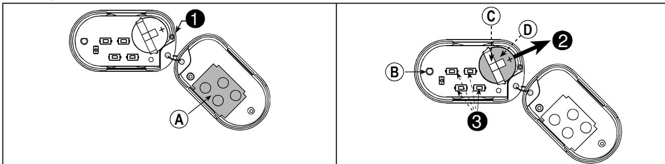
1. Remove backside screw and open the cover.
