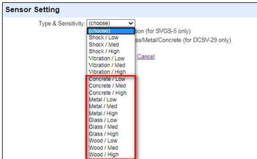
3. When DCSV-29 receives programming command from the Control Panel, the LED will first turn off, and then turn brighter and turn dark. Material & Sensitivity level setting are now complete.
