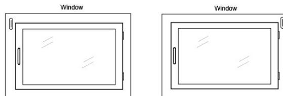
When installing on window frame, it is recommended to mount the shock sensor on the top left corner or top right corner of the window frame.
