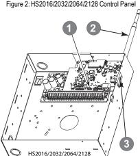
Description ltem PC-Link Cable Connector 1 Quad Band Whip Antenna - Use light pressure to attach antenna finger tight only 2 3 Screw
